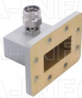
159WCANM Right Angle Rectangular Waveguide to Coaxial Adapter 4.9-7.05GHz WR159 to N Type Male
